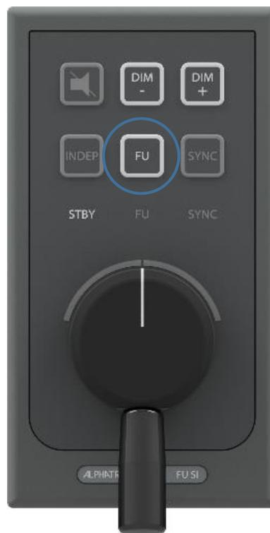
Figure 5: Enabling FU control allowed
