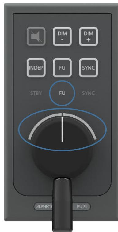
Figure 3: FU mode enabled
